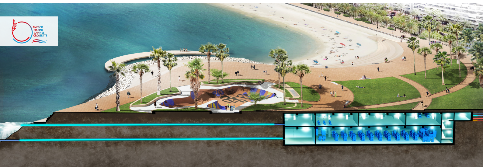
STATION SOUTERRAINE DE THALASSOTHERMIE
